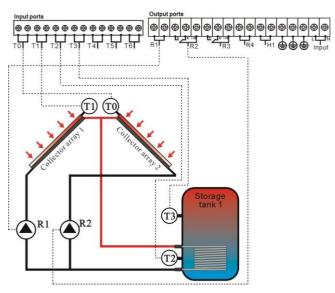
T0: Temperature sensor for collector array 2
