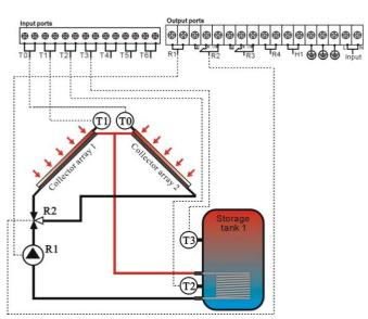
T0: Temperature sensor for collector array 2
