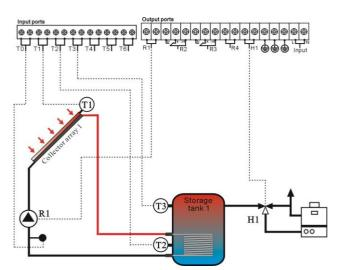
T0: Sensor for measuring the thermal energy (optional sensor)
