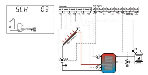
T0: sensor for measuring the thermal energy (optional sensor)
