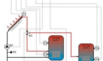
T4: Temperature sensor in the bottom part of tank 2
