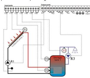
T0: Sensor for measuring the thermal energy (optional sensor)
